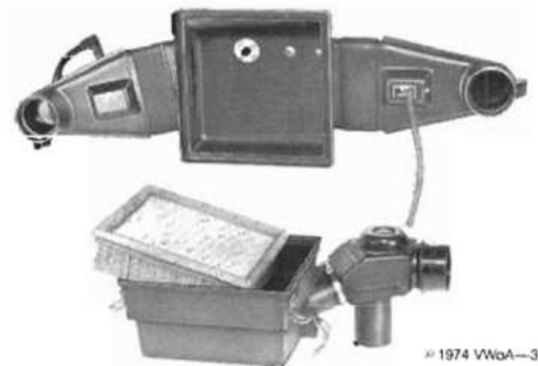
Fig. 6-3. Air cleaner with thermostatically controlled vacuum-operated flap. The thermostatic vacuum valve is located in the upper part. The valve is the part with the hose attached to it in the illustration. The diaphragm-type vacuum unit that moves the flap is in the intake of the air cleaner lower part.
