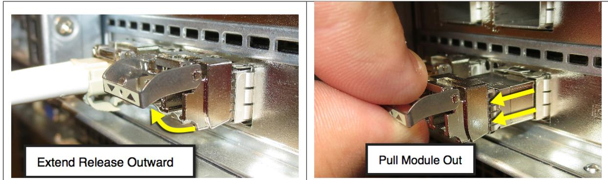
*Removing an SFP+ module*
