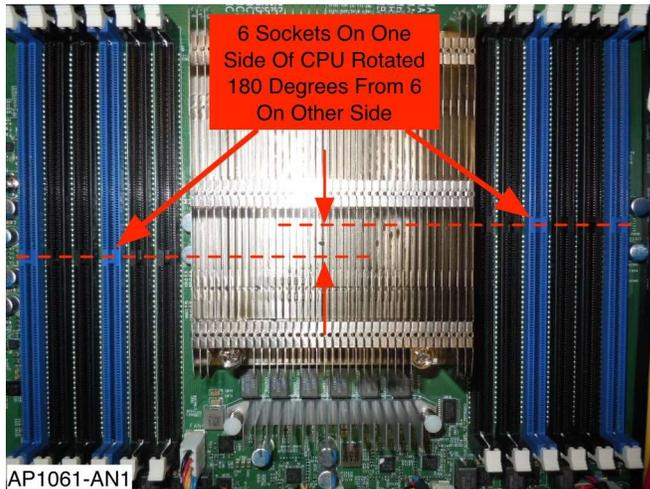
Figure 10: 180 Deg Socket Rotation Around CPU
