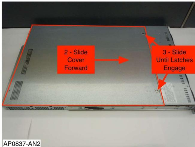
Figure 14: Installing Cover – Steps 2 and 3
