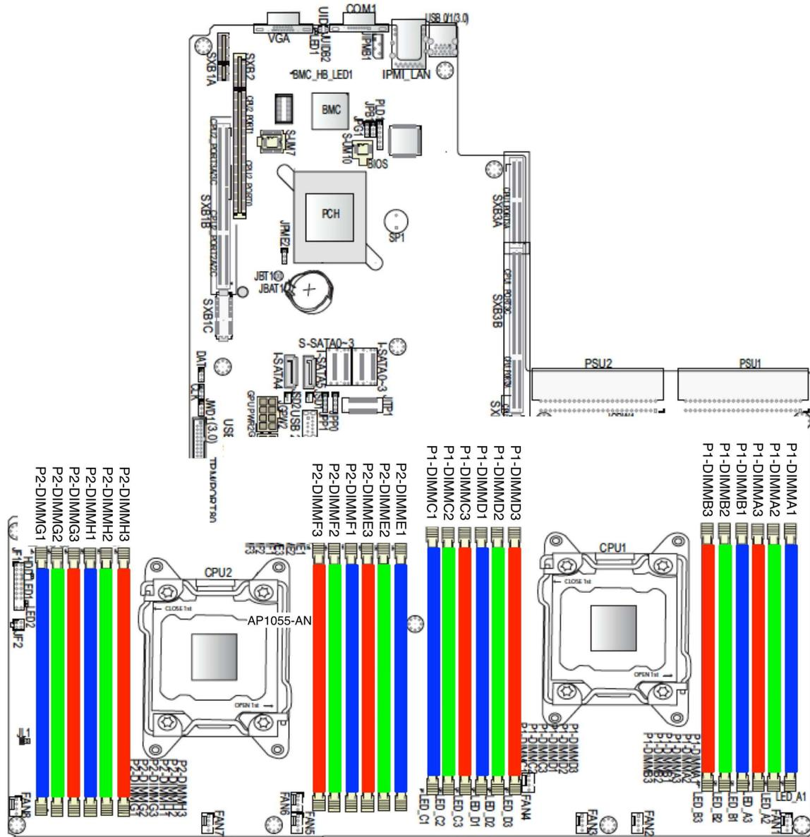
Figure 4: Motherboard DIMM Population Diagram
